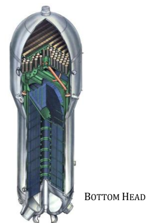
FIGURE 6A TYPICAL STEAM GENERATOR
