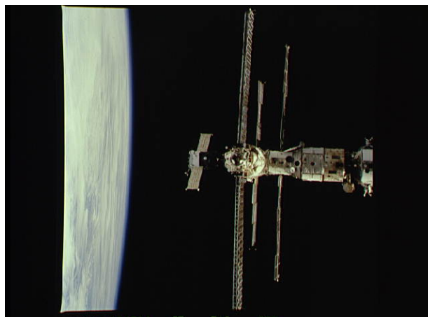
STS063-712-057 As seen from Discovery: MIR Space Station with docked Soyuz (at bottom of MIR) and Progress at opposite end.
