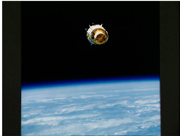
STS029-78-003--- IUS / TDRS-D after deployment from Discovery
