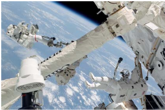
STS112-326-033 --- Wolf (left) & Sellers during 2nd EVA. Wolf is anchored to a foot restraint on ISS's Canadarm2 while Sellers traverses along the airlock spur.
