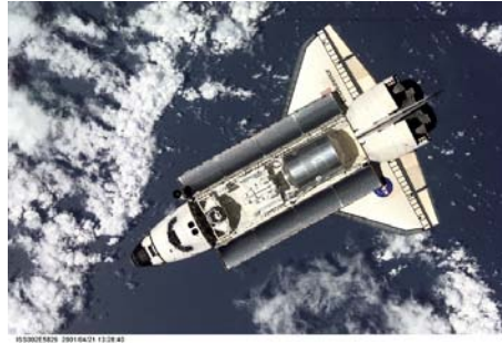
ISS02-E-5829 (21 April 2001) --- Endeavour, with MPLM Raffaello & Canadarm2 on board, approaching ISS for docking.
