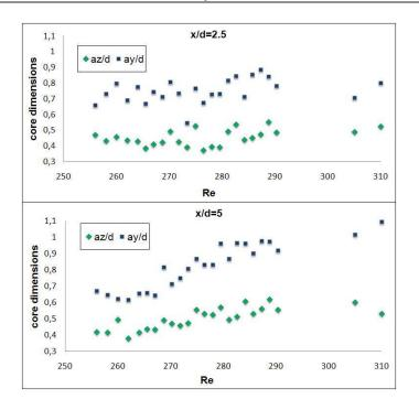
FIG. 6. Core dimensions in 2 different positions: 2.5 and 5 diameters downstream from the center of the sphere.
