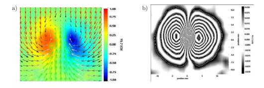
FIG. 4. a) Streamwise vorticity field in 2.5 diameters downstream from the center of the sphere for Re = 260, b) Streamwise vorticity contours in 2.5 diameters downstream from the center of the sphere for Re = 260.
