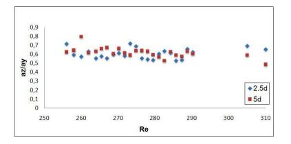
FIG. 8. The ratio of horizontal to vertical vortex core dimension as a function of the Reynolds number.
