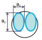
FIG. 7. The proportion of vortices' cores dimensions to sphere diameter for Re = 260.
