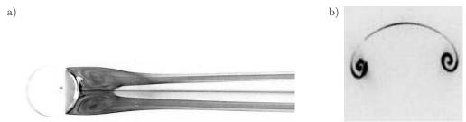
FIG. 2. Two steady counter rotating vortices – top (a) and back (b) view for Re 250.
