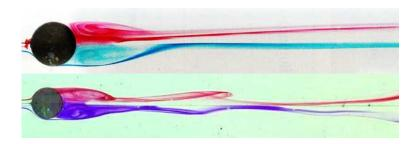
FIG. 9. Visualization with two different colours of steady and unsteady wake. Dye is fed to the flow 10 diameters upstream from the center of the sphere.
