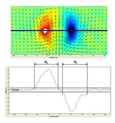
FIG. 5. Streamwise vorticity plotted on the horizontal line crossing the maximum vorticity.
