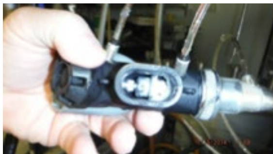
Figure 8. Regulator fitted with thermister probes.
