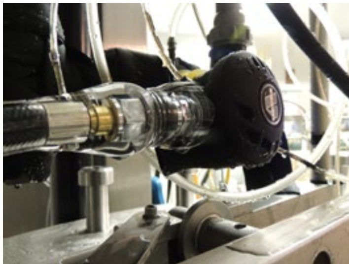
Figure 5. Ice formation on air supply line to second stage regulator
