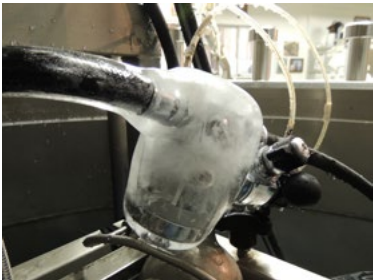
Figure 7. Extreme First Stage icing event.
