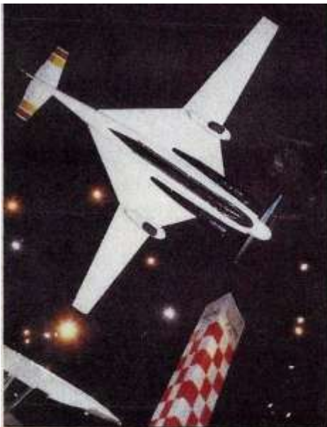
The American Special Formula One in the EAA Air Adventure Museum. Its wing planform and other features set it apart from other racers. The streamlined belly tank was used in the CAFE 400.
