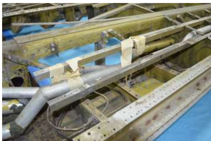
N13Y Radiator/Oil Cooling Tubing in Wings
