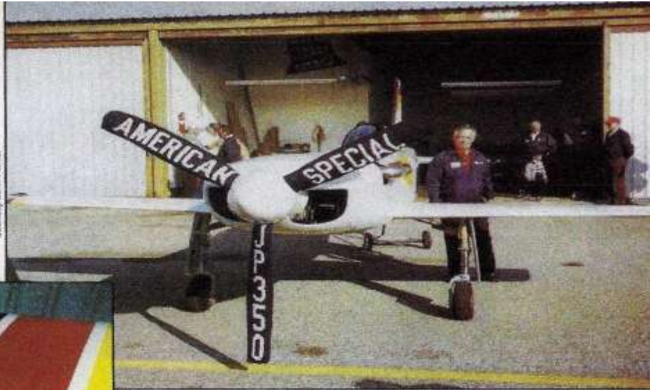
The JP-350's 18.5 ft. span is awesomely evident in this shot (top), as well as the lack of prop clearance.
