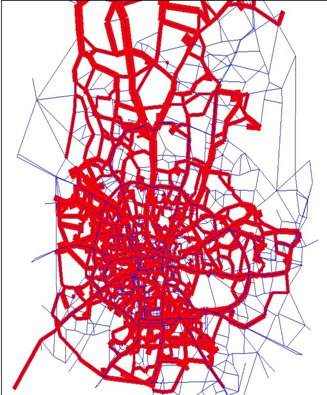
Figure 3.11 Expected Peak Hour traffic Volume (other than PT) on Road Network in 2041 with Phase I & II Scenario
