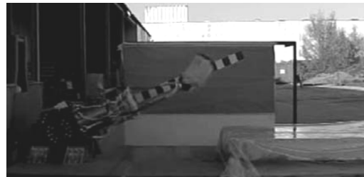
Fig. 13: Parachute dynamic extraction test
