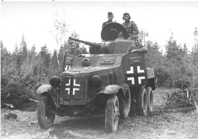
Above: Typical Russian BA-10 put back in service with German forces as the Ba-203(r).
