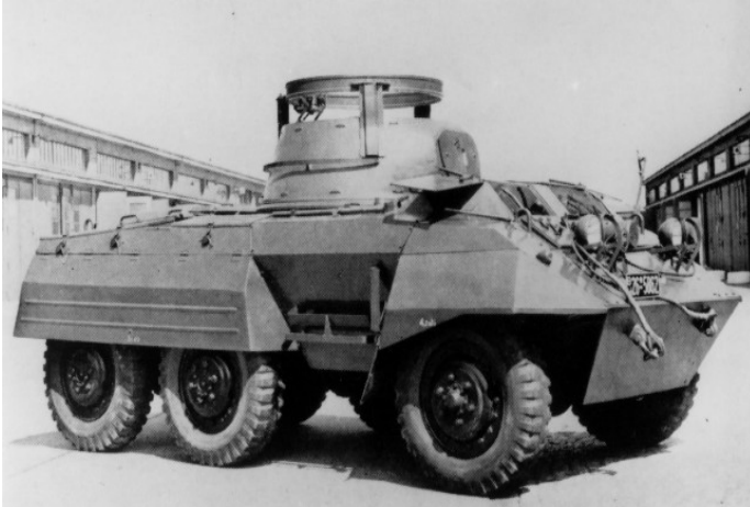
Above: M8 Greyhound with 37mm cannon removed and converted to a border patrol vehicle. Photo: Author's collection.
