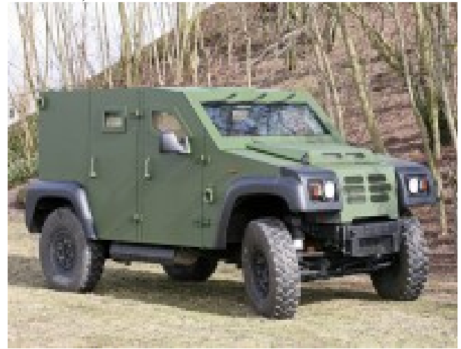
Above: Rheinmetall/Panhard Gavia under trials, this vehicle doesn't yet mount the WS 609L remote controlled weapons station. (Photo: Rheinmetall Landsysteme)
