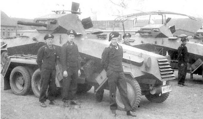
Above: Pre-WWII SdKfz 231 six-wheeled reconnaissance vehicle.
