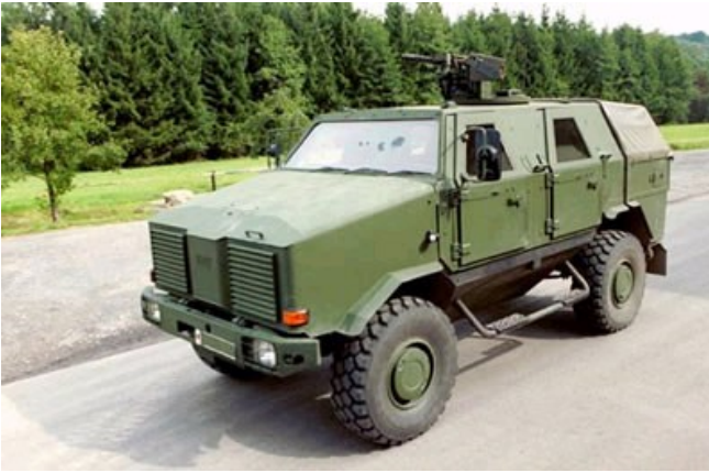
Above: This Dingo-1 has been up-graded with a remotely operated weapons station. (Photo: Krauss-Mafei Wegmann GmbH)
