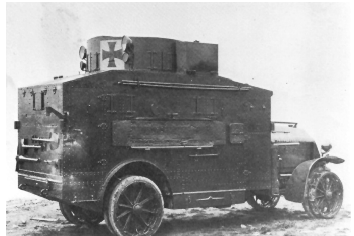
Above: The single Daimler M1915 as received by the German Army. (Photo: Daimler-Benz)
