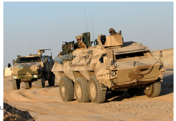
Right: A Germany Army Fuchs in support of ISAF in Afghanistan circa 2010. Immediately behind is a German Army Dingo 4x4 APC. (Photo: ISAF)
