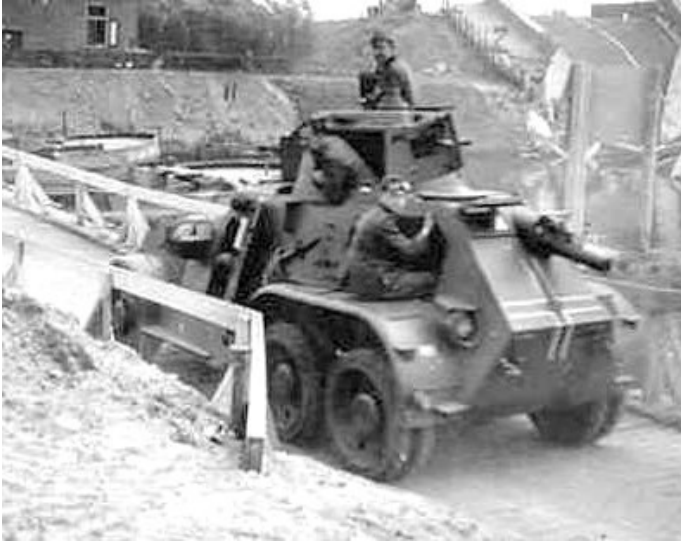
Above: Dutch M38 (PzSpw L202) captured and put into German service. (Photo: Author's Collection)
