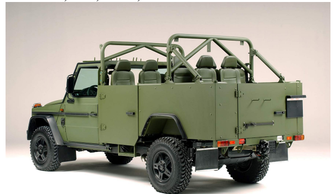
Above: Wolf ESK/LIV with passenger module. (Photo: Rheinmetall Landsysteme)
