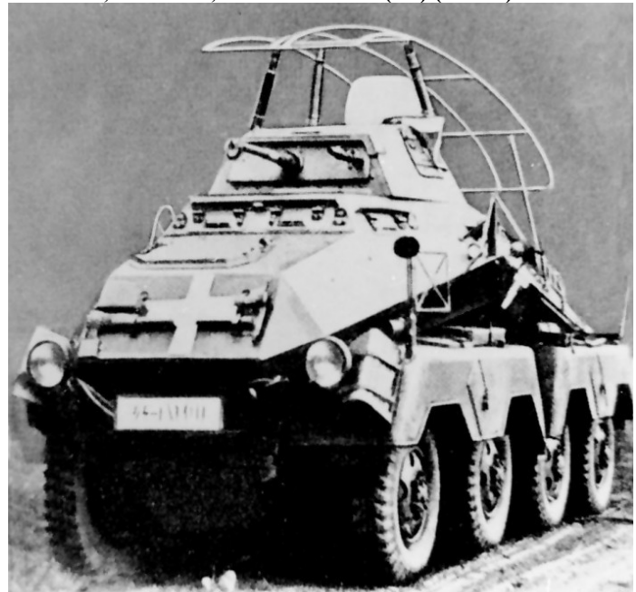
Above: A 232 with the Waffen-SS carrying a frame antenna. Some vehicles also included a telescoping high power antenna on the rear deck. (Photo: Author's Collection)
