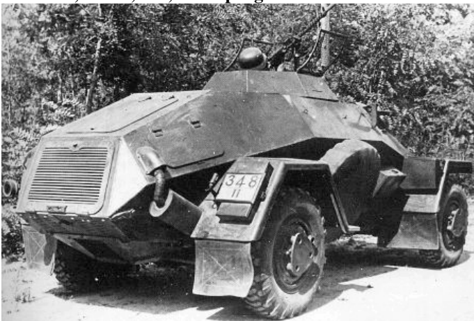
Above: SdKfz 231 (8-Rad), the vehicle was able to cross a ditch up to four feet one inch (or 1.24 meters) wide. (Photo: U.S. Army)
