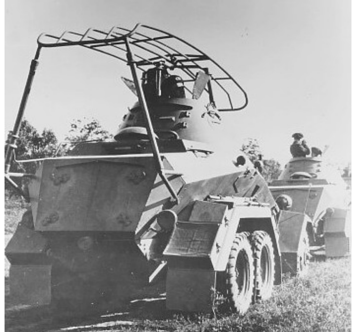
Above: The early SdKfz 232 six-wheeled reconnaissance and radio car. (Photo: National Archives)
