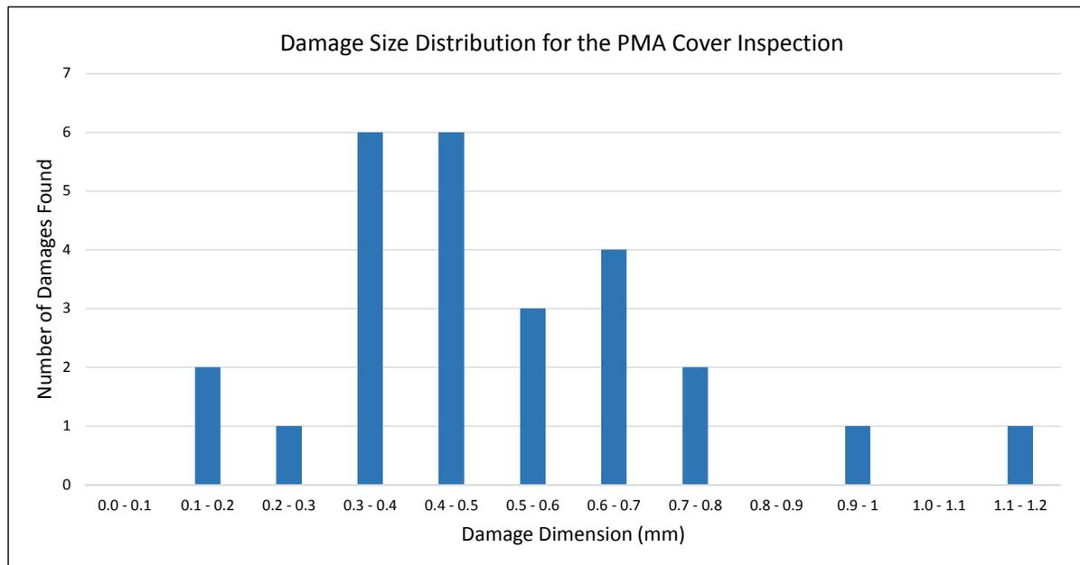
Figure 6. Damage Size Distribution for the PMA cover inspection. The number of damages found in each size bin is given in this graphic (for instance, six damages that were greater than 0.3 mm but less than 0.4 mm were found).
