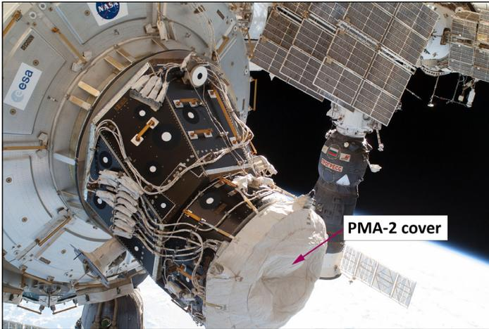
Figure 1. The cover was exposed to MMOD for 1.63 years at the forward end of PMA-2.
