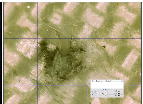
Figure 5. An impact damage (no.13) that was found on one of the hold-down straps. This damage is shown in front-light on left, back-light in middle, and through the microscope on right. The hole diameter in the outer beta-cloth layer was 0.75 mm although the dark zone in the back-lighted photo extended well beyond the hole dimensions.
