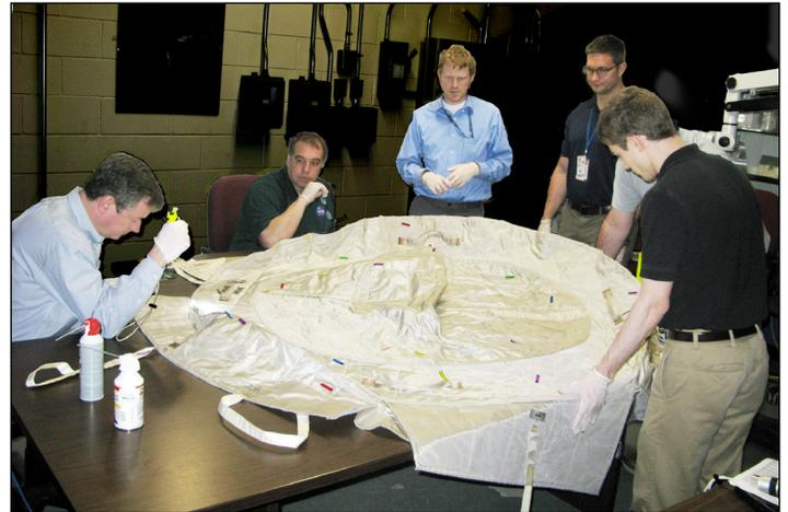
Figure 2. NASA and Boeing personnel inspected the cover for visible damages and located 26 likely MMOD impact sites.
