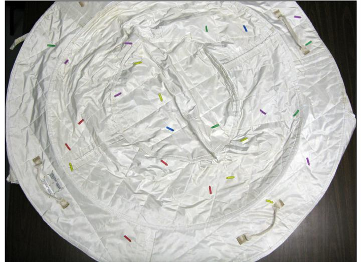
Figure 4. An overview of the cover including small labels indicating the location of each impact damage found in the inspection.
