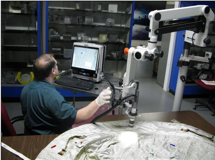
Figure 3. A 3-D digital scanning microscope mounted to an adjustable arm was used to photograph and measure the damage.
