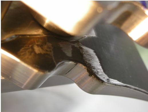
Figure 8, wear pattern on parapet duckbill
