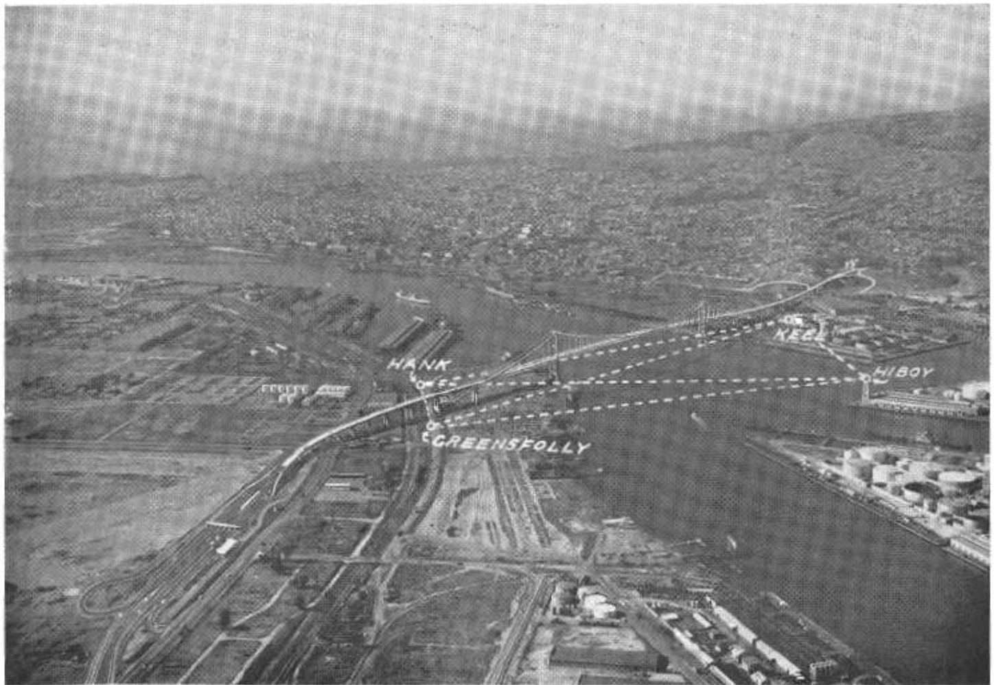
Looking southwest at the site of the future San Pedro-Terminal Island Bridge showing locations of precise control survey stations.
