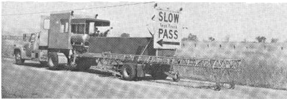
Figure 5. Traveling Deflectometer: In the recording cycle the probes and their traverse assembly remain stationary on the road while the truck moves forward.
