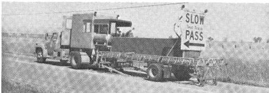
Figure 6. Traveling Deflectometer: The traverse assembly is picked up by a pneumatic operated track and carried ahead and dropped on the road to repeat the cycle.
