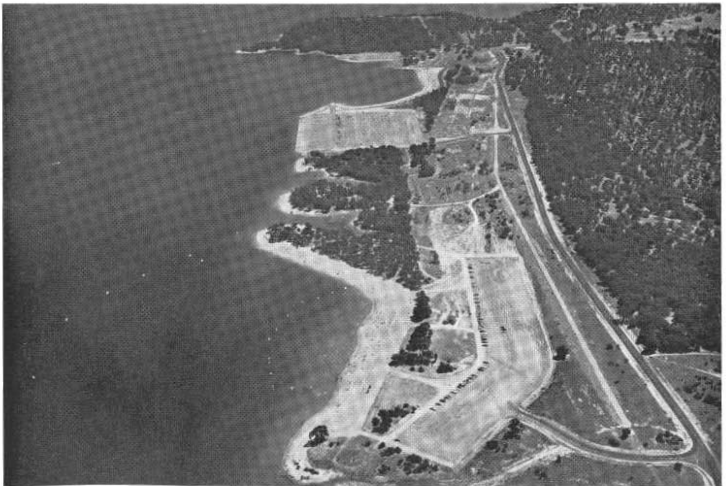
Looking south at Granite Bay facilities during near high water mark in June. This year's improvement of the swimming area (lower center) extended usable beach by placement of local decomposed granite below the visible beach in the photo to an area roughly bounded by the outer ring of buoys making the former rugged, rocky surface safer and more usable during low water. Entrance and connector roads, some ramps and initial beach were constructed for the Division of Beaches and Parks in 1958 under a Division of Highways contract.
