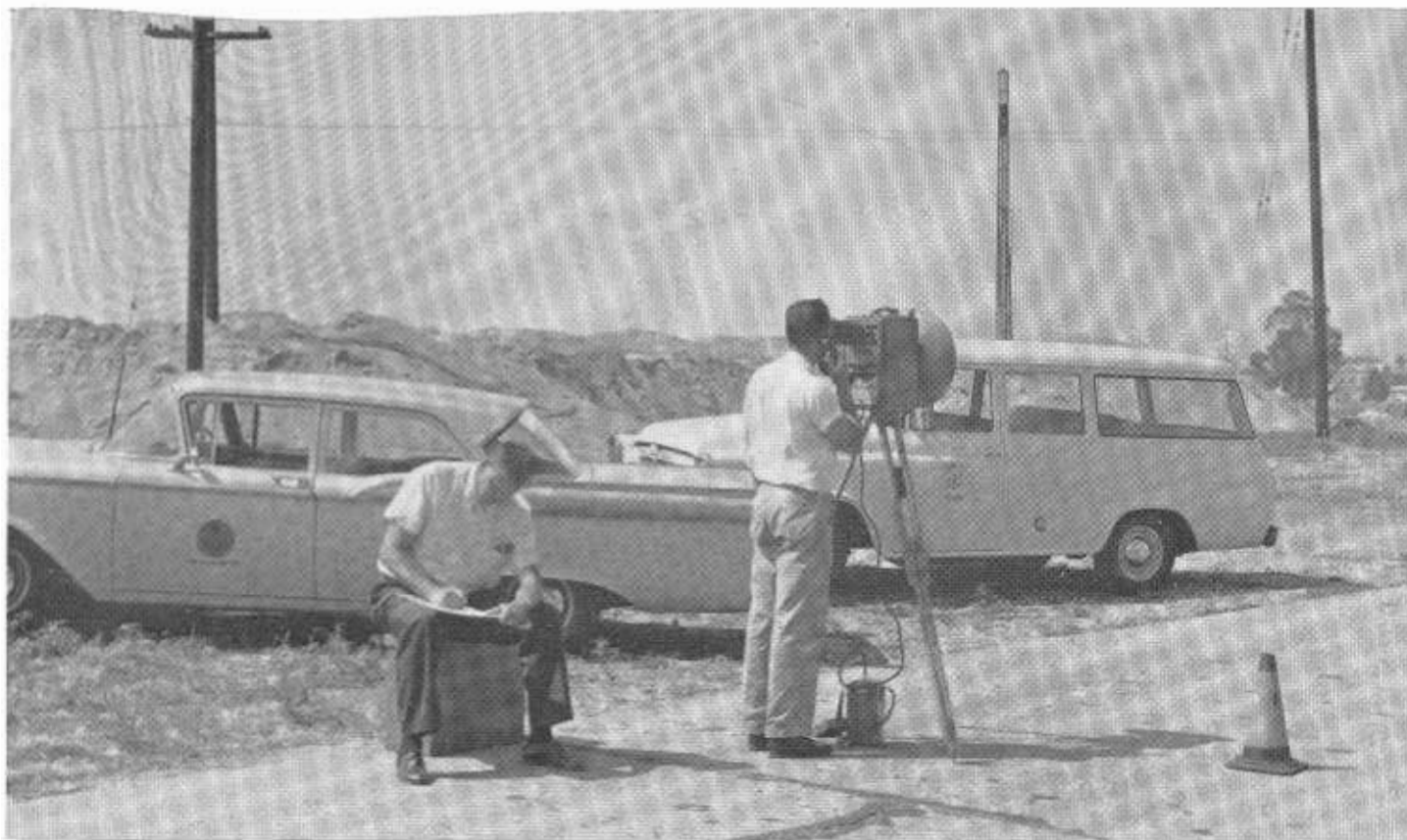
Bob Barron of Los Angeles City Engineering Department operating Tellurometer. Al Whitlock of State Division of Highways recording at Station "Keel."
