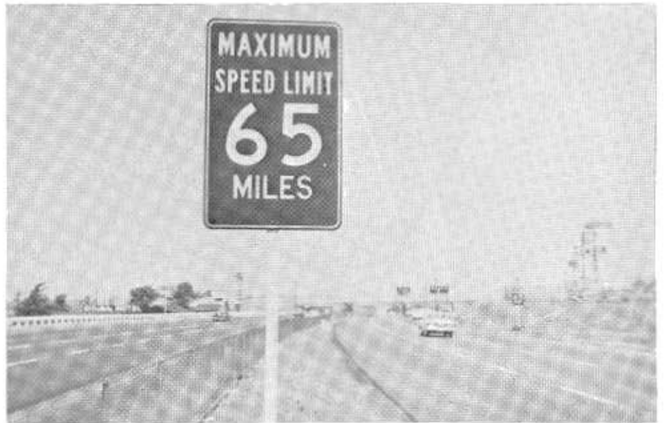
Speed limit signs are the most familiar examples of regulatory type sign.
