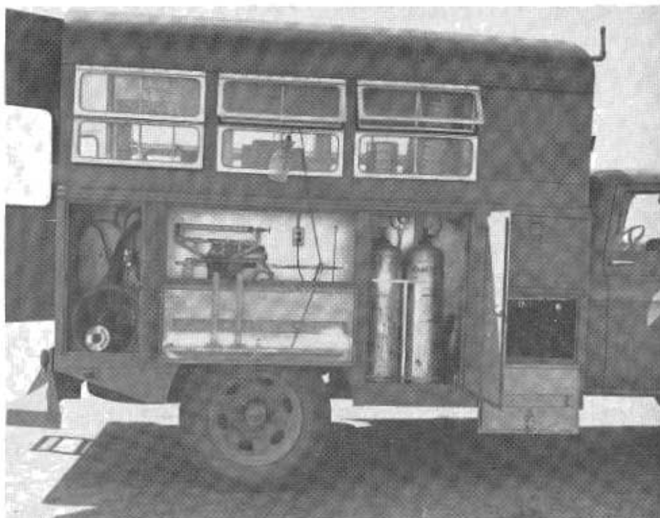
View of right side of mobile laboratory with compartments open, showing air compressor, butane tanks, sand equivalent test area and equipment, and storage for hoses and electrical cords.
