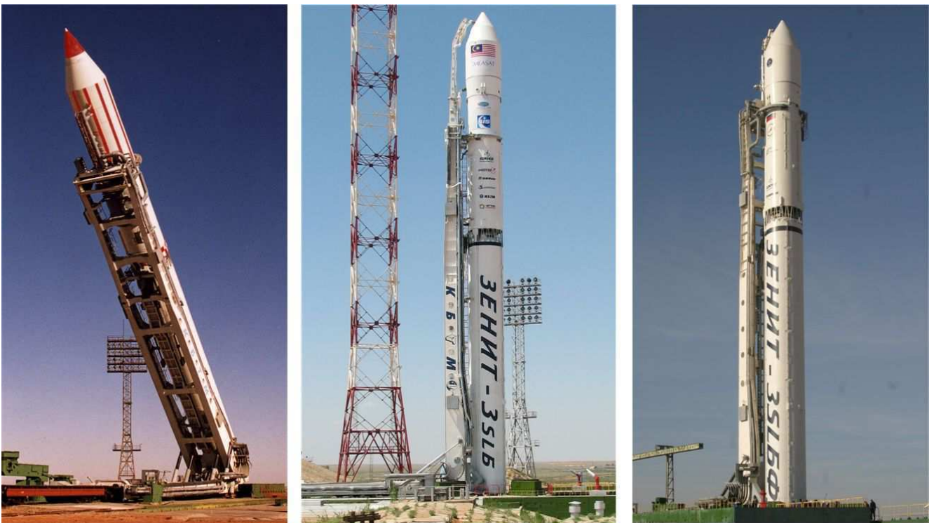
Figure. Three configurations of the Zenit family vehicles (left to right): Zenit-2SLB, Zenit-3SLB, Zenit-3SLBF
