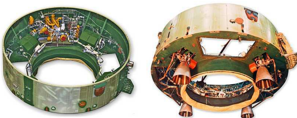
Figure. Second stage aft bay
