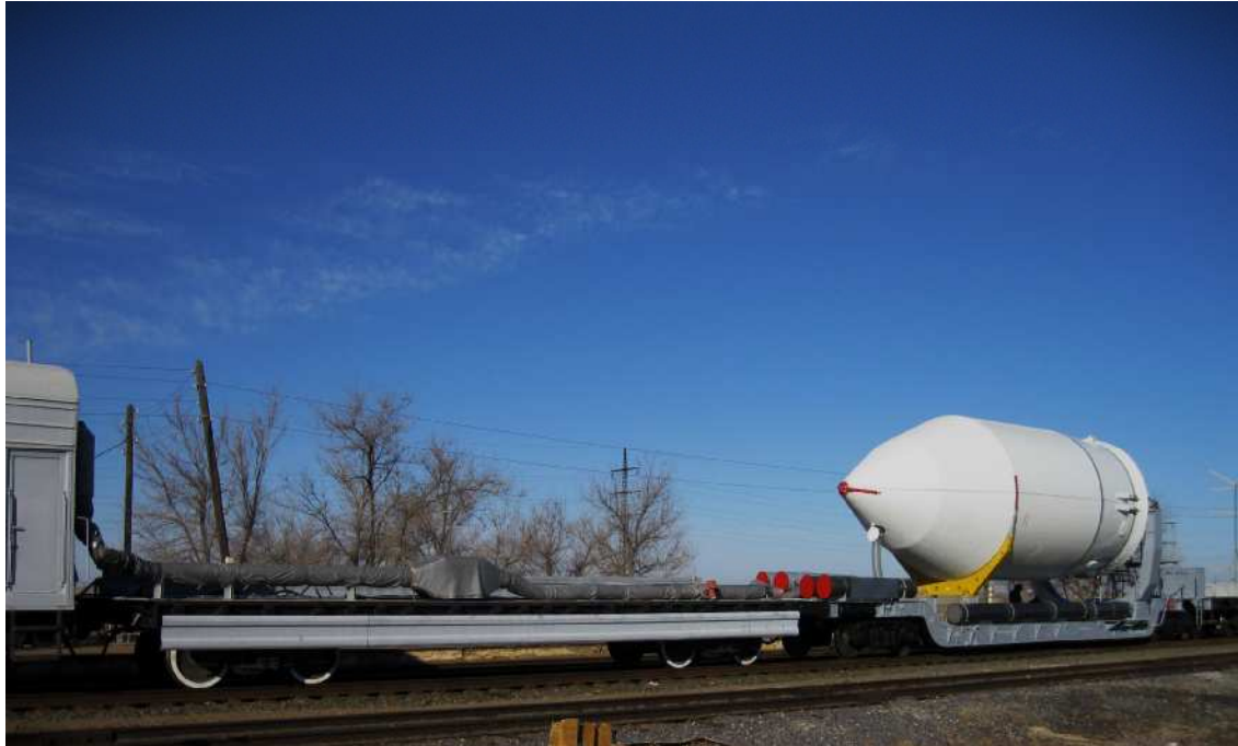
Figure 6-5. Transfer of Zenit-3SLBF Ascent Unit with thermostating wagon
