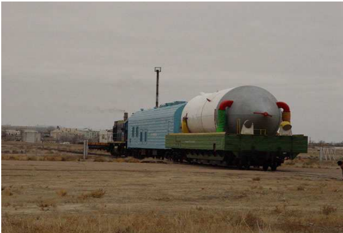
Figure 6-4. Transfer of Zenit-3SLB Ascent Unit with thermostating wagon
