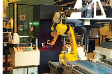
Automatic appearance inspection by the iRVision
