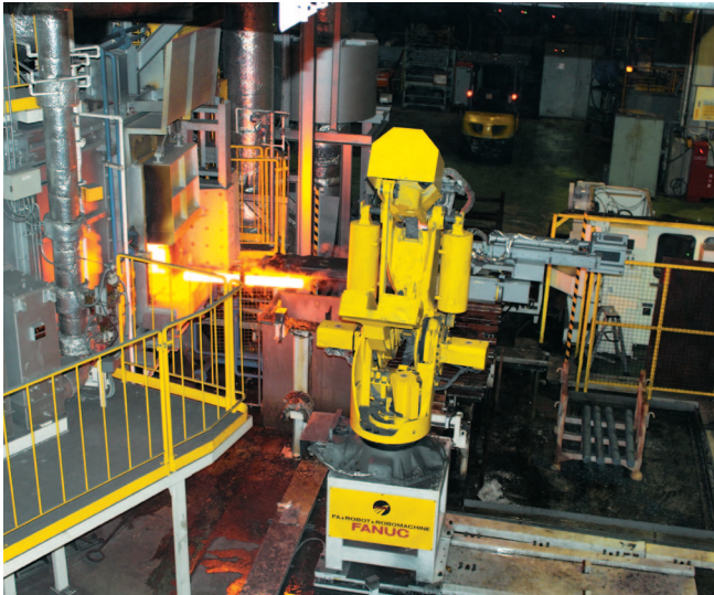
Robot picking parts from a rotary furnace
