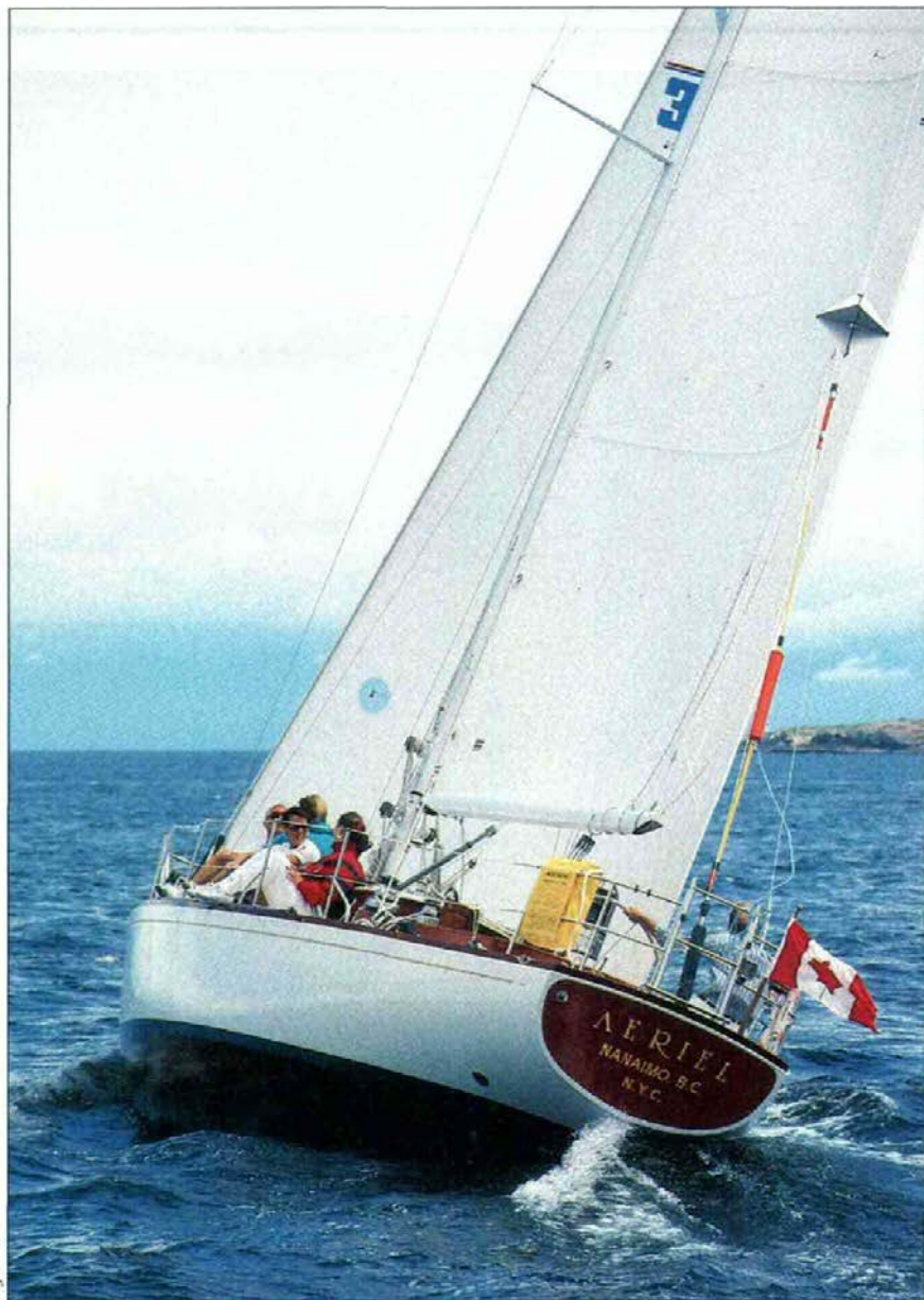
AERIEL, unlike her predecessor (designer Jim McCurdy's SELKIE), carries a traditional aft-raked transom.
