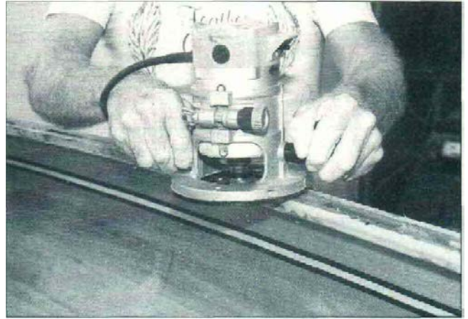
31. Use a router with a 1/2"-round over bit on the rails, deck, and thwart. If you have no router, a plane will do. Follow up with a dual-action sander. Prepare, and 'glass the decks the same as you did the hull. Make sure the underside of the deck is well sealed with epoxy.
