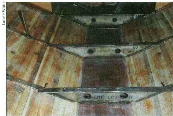
Seven bronze floors are bolted and bonded athwart the keel. Two are bolted to bulkheads, and the others attach to berthfaces, creating a longitudinal girder.
