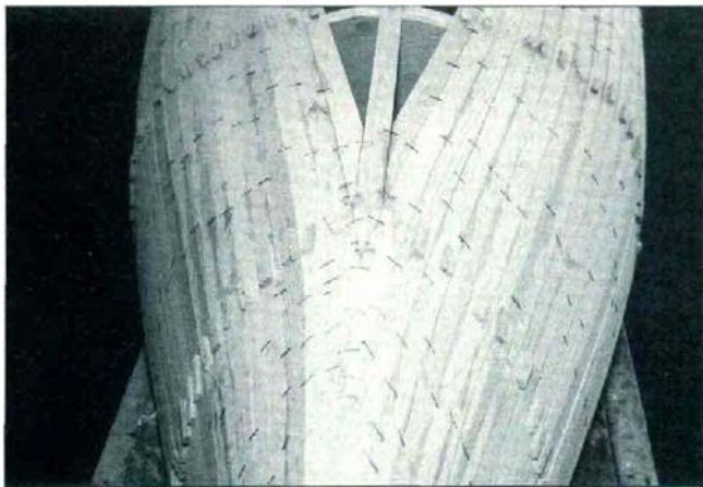
15. This photo shows how I handle the transition from stem to keel line. By running a center keel strip, you can control the fairness of the keel area. Without it, butting strip to strip, you can end up with a very unfair keel line. Cutting the strips into the keel strip takes time and care. I do as much of it as I can with the table saw, and the rest with the Dosuki saw, right on the boat.
