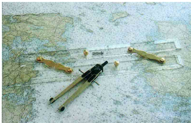
The Weems and Plath Ultralight model #176 dividers, and the 15" model #142 graduated parallel rules.
