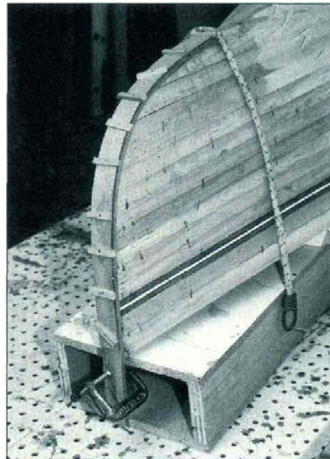
16. After trimming the strips flush with the inner stem, I laminate thin (1/16") strips of mahogany or cherry to make an outer stem. I use the same thin nails I used to hold the strips to the molds. Clamps and shock cord will help. Let this set up overnight.
