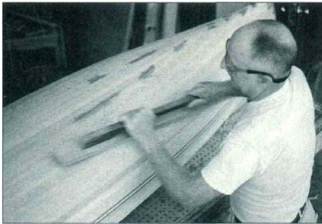
20. No matter how good you are with the disc sander, board-sanding is the best way to make sure that the hull is fair. The abrasive paper that auto body shops use on airfiles is just right for this. The process is good exercise, and it doesn't create the dust that power-sanding does.
