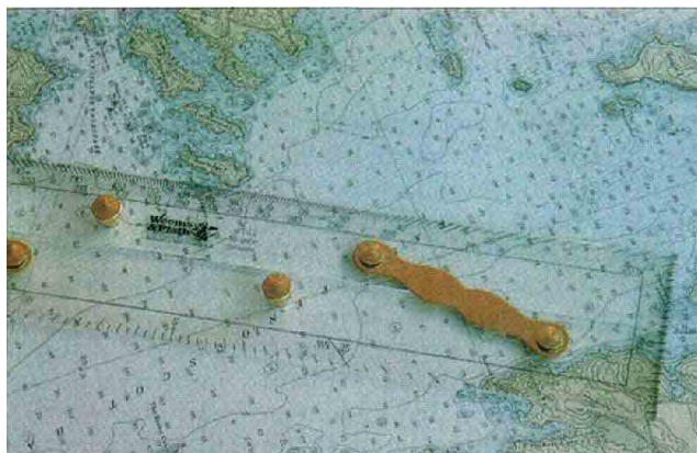
The "base" rule is shifted so that the "S" mark lies directly on the meridian, and the rules are closed. The protractor reads the course true where it intersects the meridian. In this case the course is either 27CP or 030 T.
