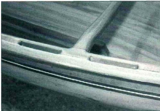
32. This is a detail of the finished thwart and rails.
