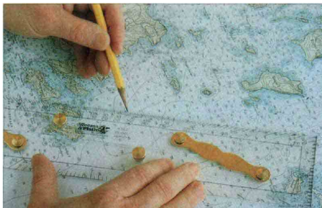
The course line is drawn as necessary, and the parallel rules are placed so that a meridian is as close as possible to the "base" rule.
