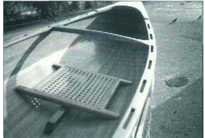
33. The seat support is epoxied in place along the centerline. Two screws hold the caned seat to the support. I do not anchor the ends of the seat frame, as this sets up stress when someone really heavy drops into the boat.
