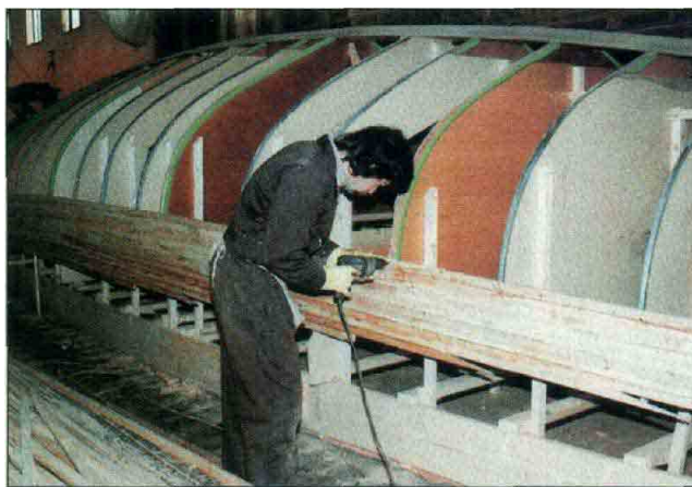
The hull was first strip planked over molds and permanent bulkheads. The two main bulkheads are foam-cored; the others are solid ply.
