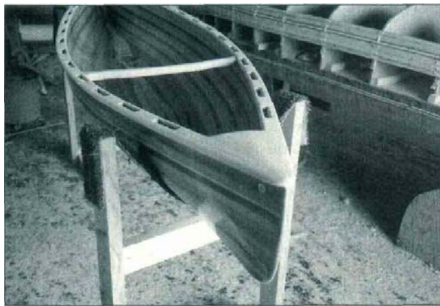
34. Now sand everything in preparation for varnishing. I use about three coats of a good spar varnish to protect the epoxy from ultraviolet rays.
