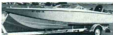
Mongoose — 19'8"; 86" Beam; Deep V Racer; Speeds over 60 MPH with 200 hp; Excellent for Racing or Skiing; Plans & Patterns $58; Hull Kit $1,775; Boat Kit $2,385. #KS 198 (cuddy cabin version available)
