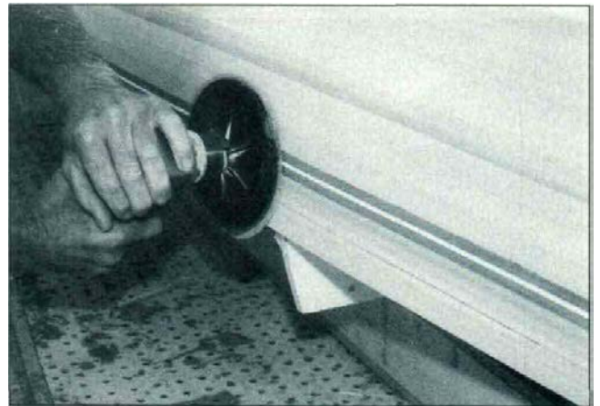
21. After board-sanding, finish with a dual-action sander. I have a Porter Cable variable-speed with a contour disc that does fine. Start with 40-grit, and follow up with 80-grit stick-on discs. Be sure you wear a face mask.
