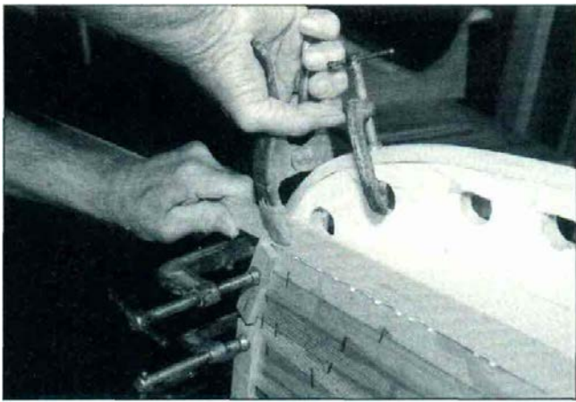
13. As the bends become tighter, use clamps to help hold the strips at the stems, until the glue sets. You have four or five difficult strips on a Wee Lassie, then the pressure eases off.
