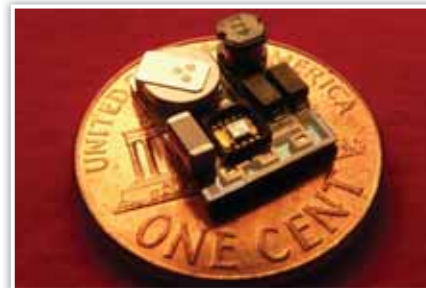
This energy harvester reaps power from vibrations.
