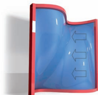
Figure 5.42: Case 1: All edges restrained with horizontal load
