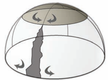
Figure 1.10: Pressure and tension in sphere shaped shell
