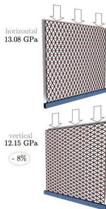
Figure 5.26: Influence of the member orientation on the total generated Von Mises stress
