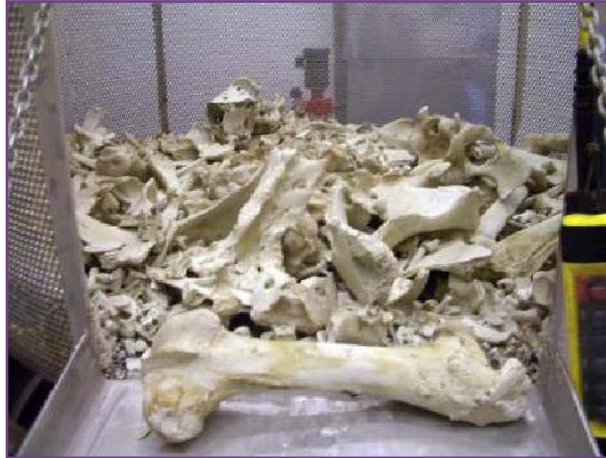
Figure 3. The crushable bone and teeth remaining from a carcass digester in a fixed alkaline hydrolysis facility. (Photo courtesy of Waste Reduction by Waste Reduction Inc., Indianapolis, IN)
