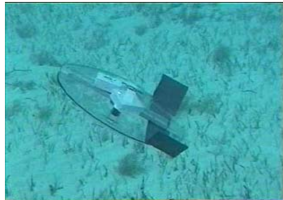
Figure 7b – Model Discus Glider in salt water ( 45^{\circ} wings)
