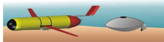
Figure 1 – Cylindrical glider vs. Lenticular glider resting on bottom sediment
