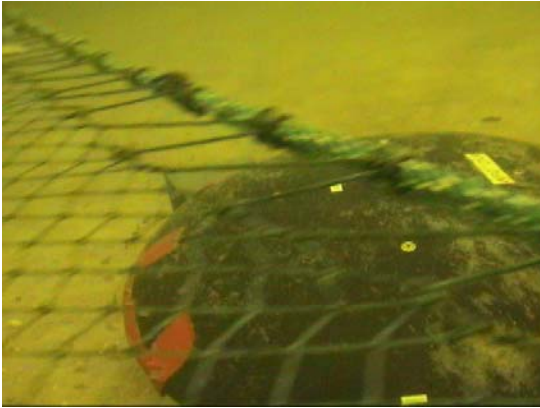
Figure 8 – Trawl net passing safely over WRC Discus Glider
