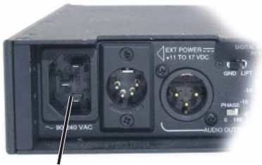
AC Power Input Jack 90 to 240 VAC, 50-60 Hz
