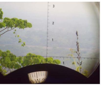
Accounting for the declination, we aimed the antenna to a bearing of 277 degrees
