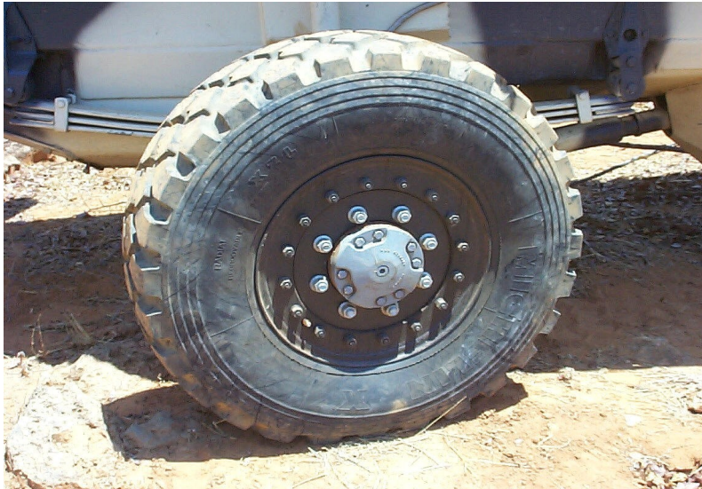
Detail of run flat tyre.
