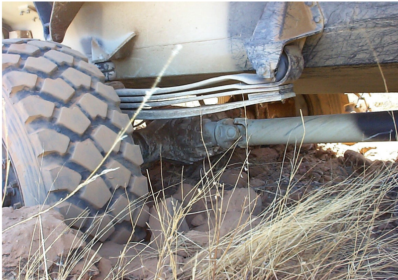
The rear wheels dug in when the front axle broke down.
