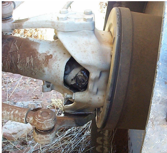
The damaged universal joint.
