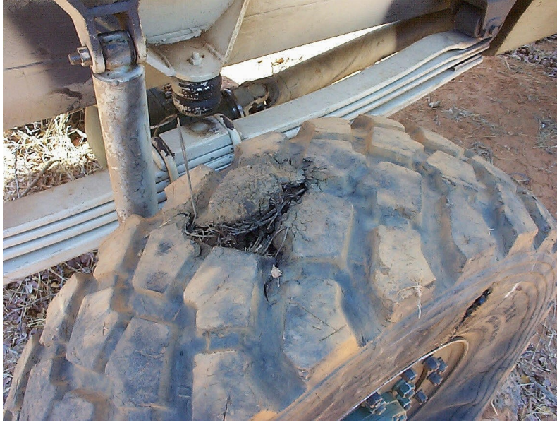
Damage to the run flat tyre after an AP mine detonation.
