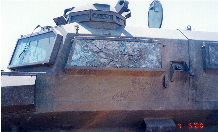
The side blast surface-cracked the windows, but no penetration occurred.
