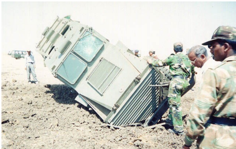
The Medak vehicle lying in the blast crater after the same test.
