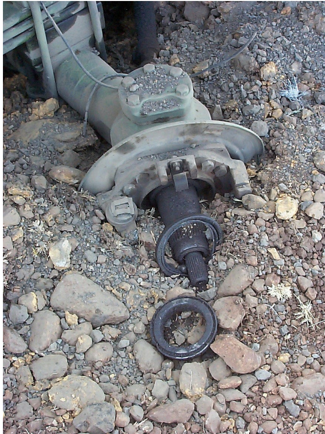
Detail of damage to right front wheel station after front axle centre blast test. The wheel with hub is blown off, but the axle is repairable.
