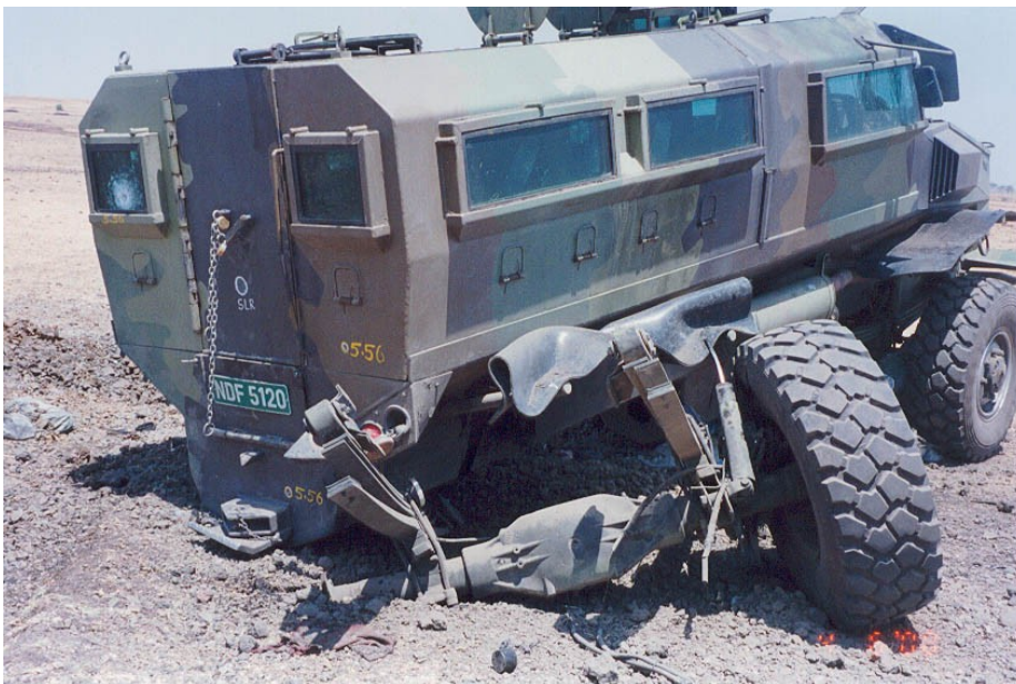
The axle is ripped out to the right rear by the blast force. The vehicle remains field repairable and there is no blast intrusion into the cabin.
