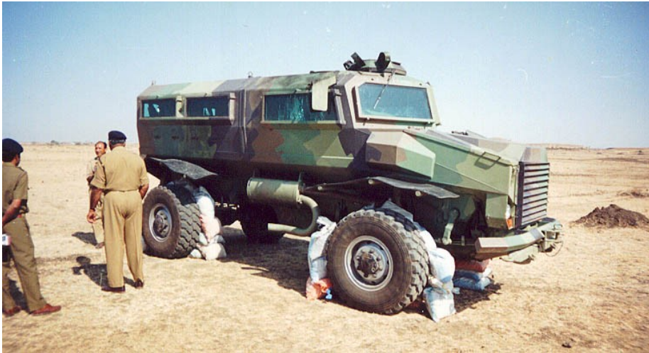
The vehicle is set up and ready for the rear wheel blast test.
