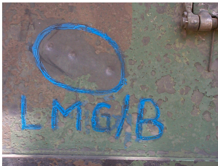
LMG burst on hull side.
