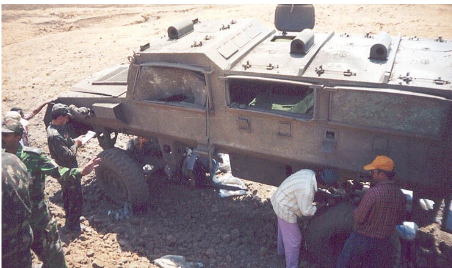
The Medak vehicle after its side blast test. The side windows are completely blown into the cabin. With the resulting pressure intrusion it is doubtful if anyone would have survived this blast.
