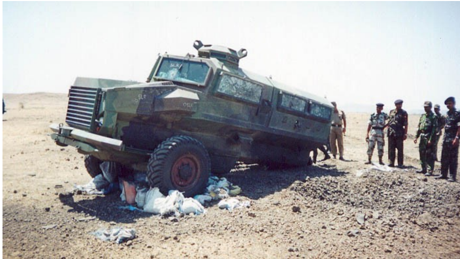
The vehicle is not thrown over by the wheel blast, nor is it moved forward. The rear end is rotated by 30 degrees to the right. Note the blast crater.
