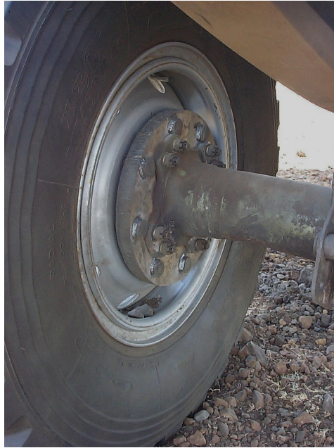
The static axle repair.
