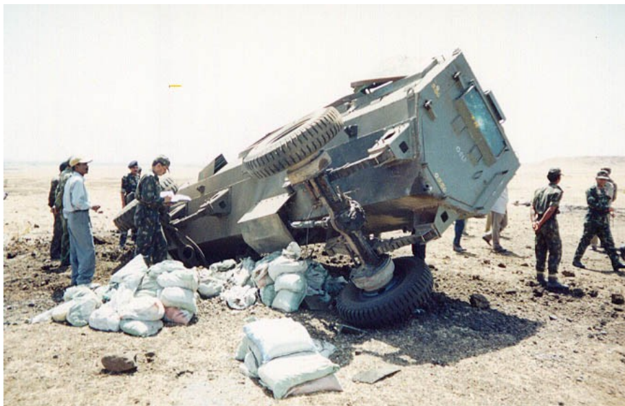
The Medak vehicle after the front axle centre blast.
