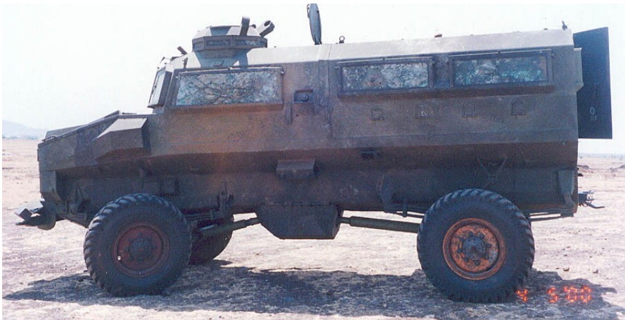
Damage after the MKII IED side blast. No pressure intrusion occurred.
