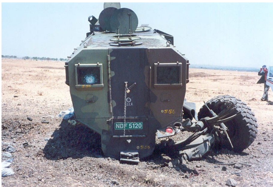
Blast results of an equivalent triple anti tank mine hit.
