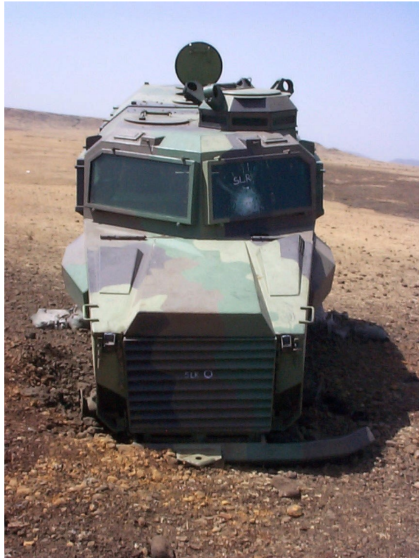
Wer'wolf MKKII lying in the blast crater after the front axle blast test.
