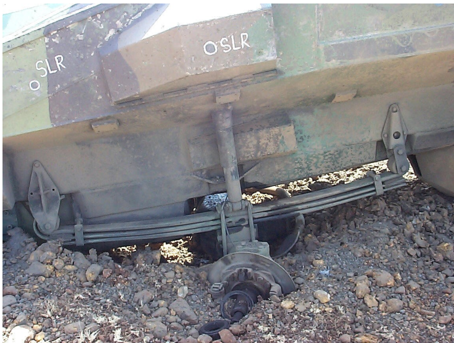
Left front view of damage after the front axle centre blast test. Note virtually no damage to the springs, hanger brackets and shock absorbers.
