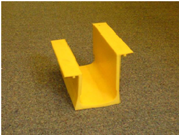
Figure 15 - Short prototype length and visualisation of the embedded rail pad
