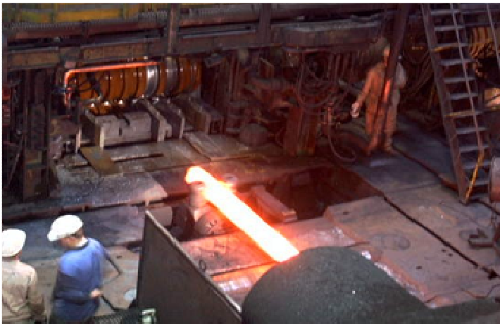
Figure 13 - Manufacture of the BB14072 embedded rail
