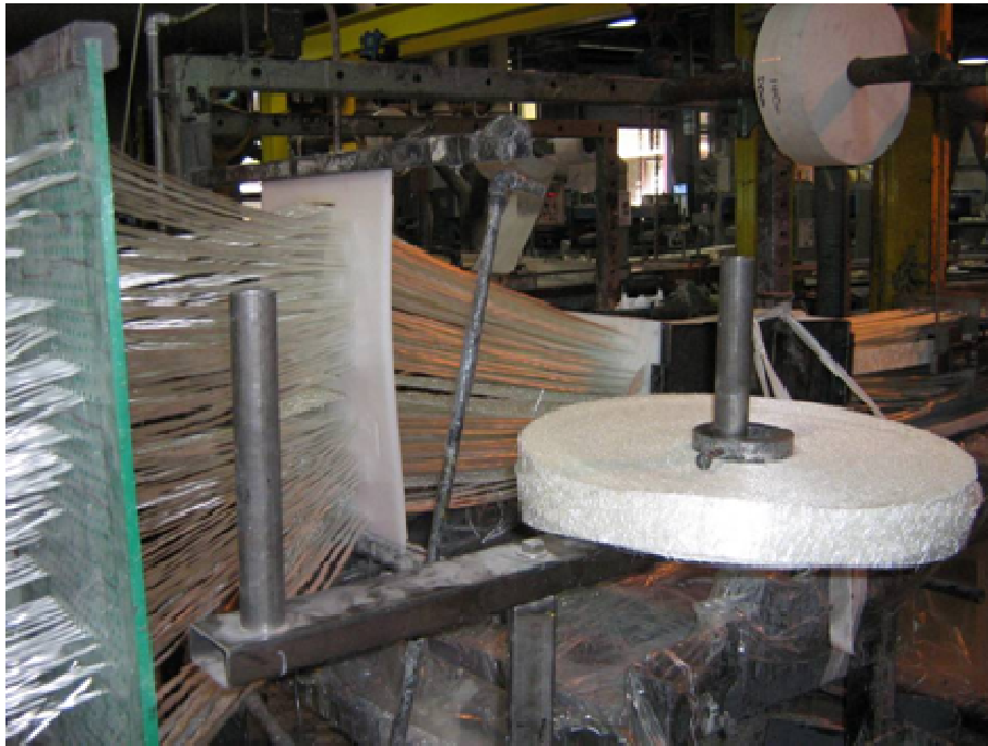
Figure 17 - Embedded rail shell Manufacturing process
