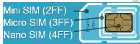
Figure 2: SIM Card Size Formats [Orm09]
