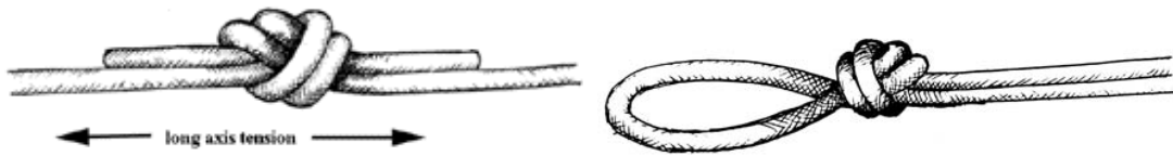
A bend and a loop stressed along their long axes - correct applications in each case
