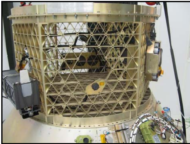
Figure 8: SPASS integrated onto launch vehicle payload adapter and ready for primary payload integration
