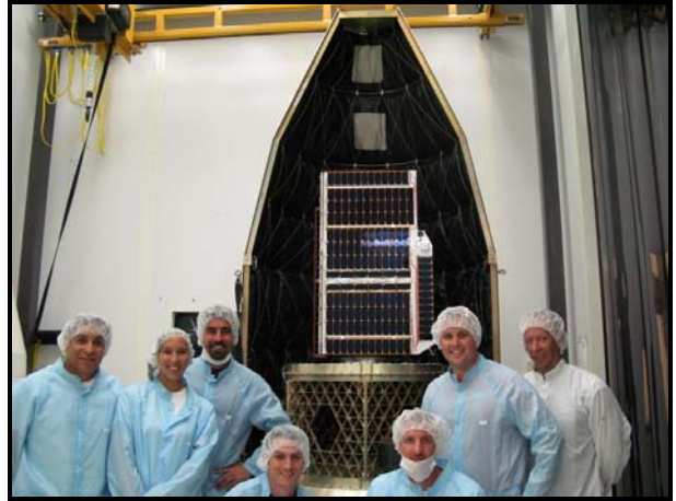
Figure 10: Jumpstart mission integrated payload stack ready for fairing encapsulation
