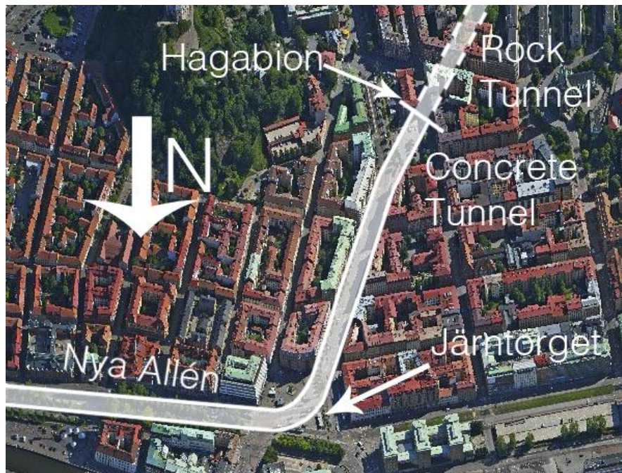
Figure 5.5 The part of Linnégatan intended for Allélänken. The geometry of the tunnel in this picture is merely a sketch and is thus not accurate (Eniro, 2012 (edited)).
