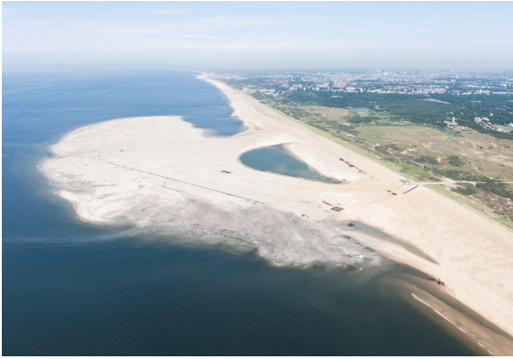
Aerial photo (June 2011) of the sand motor, a pilot project along the Dutch coast which seeks to find more sustainable means to combine beach replenishment and coastal protection.
