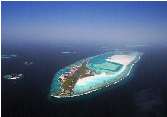
In the Maldives, new land has been reclaimed from the sea to build a new island called Hulhumale next to Male. This has relieved some of the overcrowding on Male itself.
