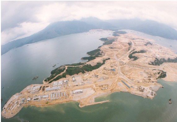
Far eastern airports in the sea include from top to bottom: Singapore's Changi (where vertical drains were used to expedite subsoil consolidation), Hong Kong's Chek Lap Kok (where a natural habitat was preserved and integrated into the land reclamation) and Japan's Kansai airport (the 2nd phase expansion is shown here).
