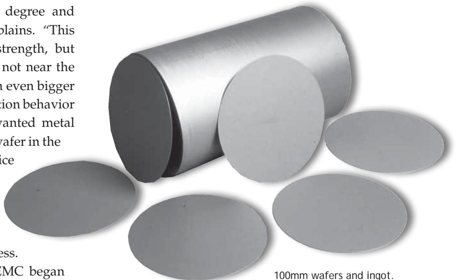
100mm wafers and ingot.
