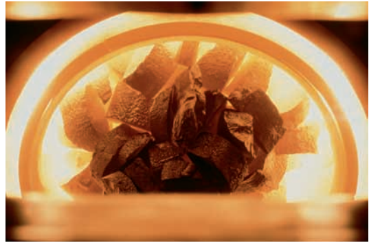
Chunk polysilicon is melted.
