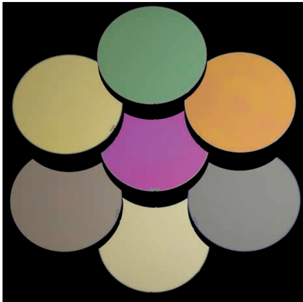
"Silicon-on-Insulator," a.k.a. SOI, wafers were originally manufactured by SiBond, LLC, a joint venture between MEMC and IBM. These wafers were produced in 2007.
