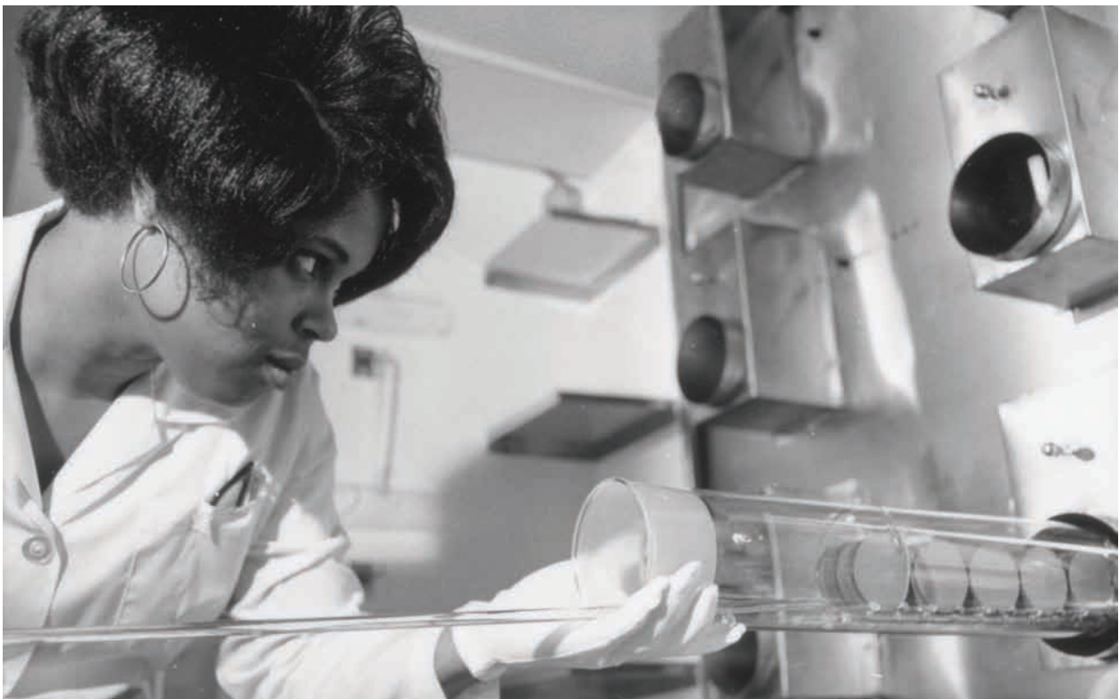
Wafers are inserted into and extracted from a warming oven, slowly allowing them to heat or cool to avoid dislocations in the crystal lattice.
