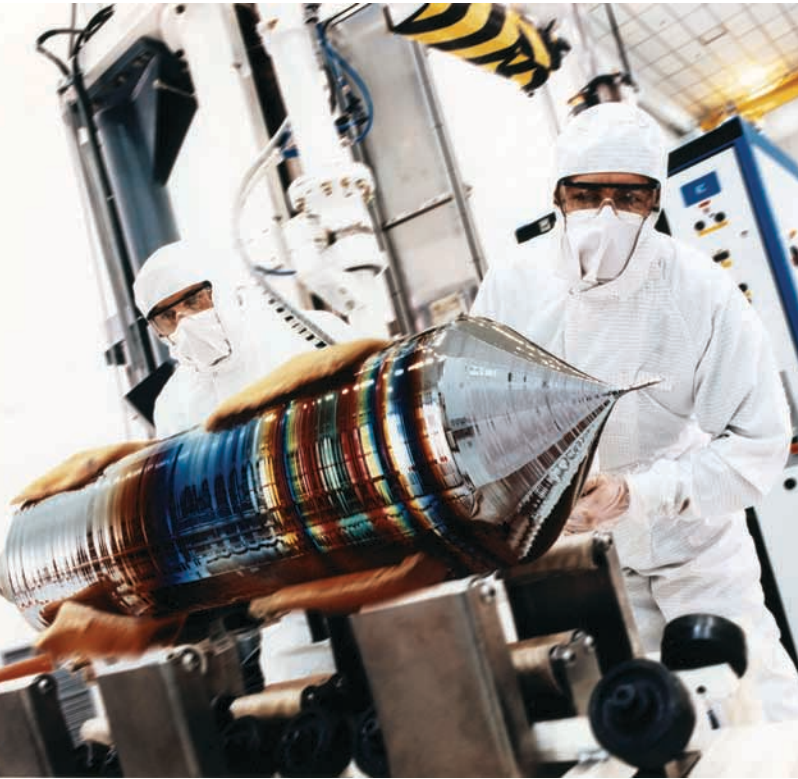
A 300mm ingot is loaded onto a cart for transporting to the next process.
