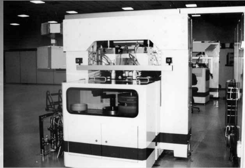
Double side wafer grinder at MEMC Southwest’s modifications area, April 1997.
