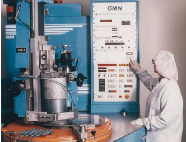
Inner diameter saw with back grinding capability, which reduced the amount of required lapping.
