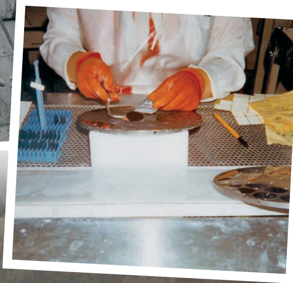
Polishing two-inch wafers.
