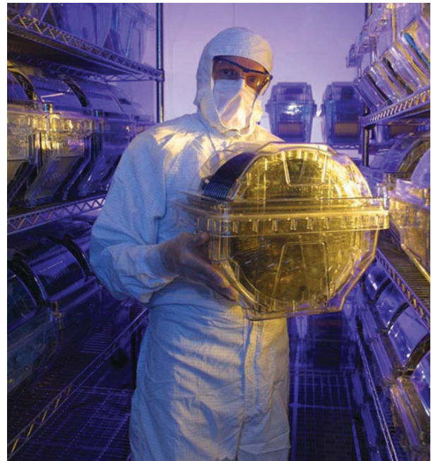
The 300mm wafers in carriers are stocked on shelves in the clean room during processing.
