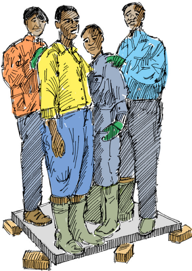
Figure 27. Testing the slab
