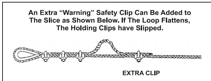
Figure 3-5. Joining Wire Ropes.
