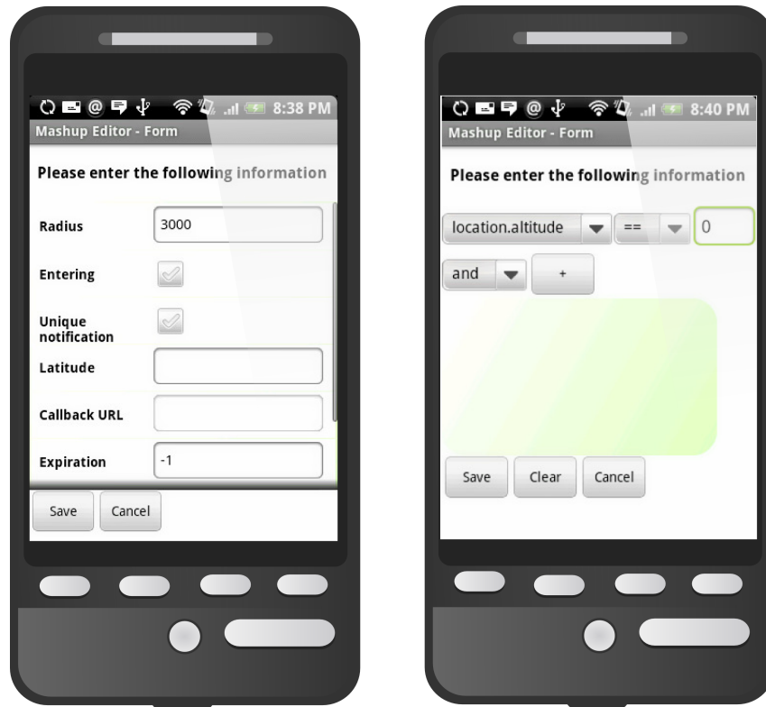
Figure 3.24: Wizard to create a mashup based on information pushed by smart things (left). The form represents the parameters that have to be provided in order to subscribe to the RESTful phone GPS proximity event (right).
