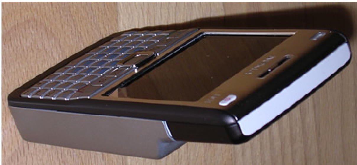
Figure 4.9: Prototype of a mobile phone extended with a UHF EPC Gen2 RFID reader. This device can read RFID tags from a distance of about 30-50cm.
