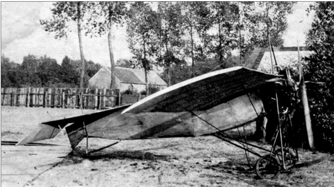
The 'new system' of control mentioned as used on the Behaeghe monoplane in 1912 appears to be wing warping.
