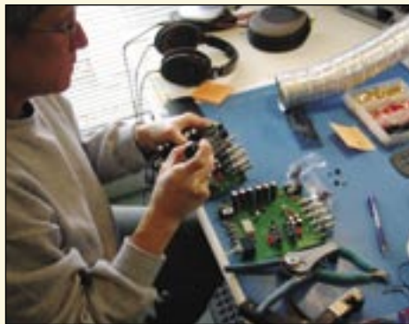
Easy-to-reach point of use storage in the electronics build cell improves work environment.
