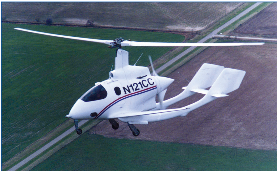
CarterCopter CCTD in flight. Developed by Jay Carter, Jr. and his associates, the state-of-the-art Carter Copter Technology Demonstrator is the most innovative rotary aircraft flying and is advancing autogyro technology to the next level. (Photo courtesy of CarterCopters, LLC)
