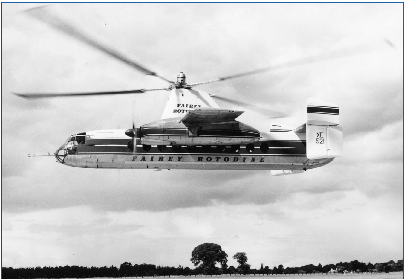
Fairey Rotodyne “Y” convertiplane, which could take off and land as a helicopter and fly as an autogyro, in a test flight during 1957-1962. It could carry 40 passengers and a crew of two and cruise at 200 miles per hour. (Photo courtesy of Westland Helicopters, Ltd.)
