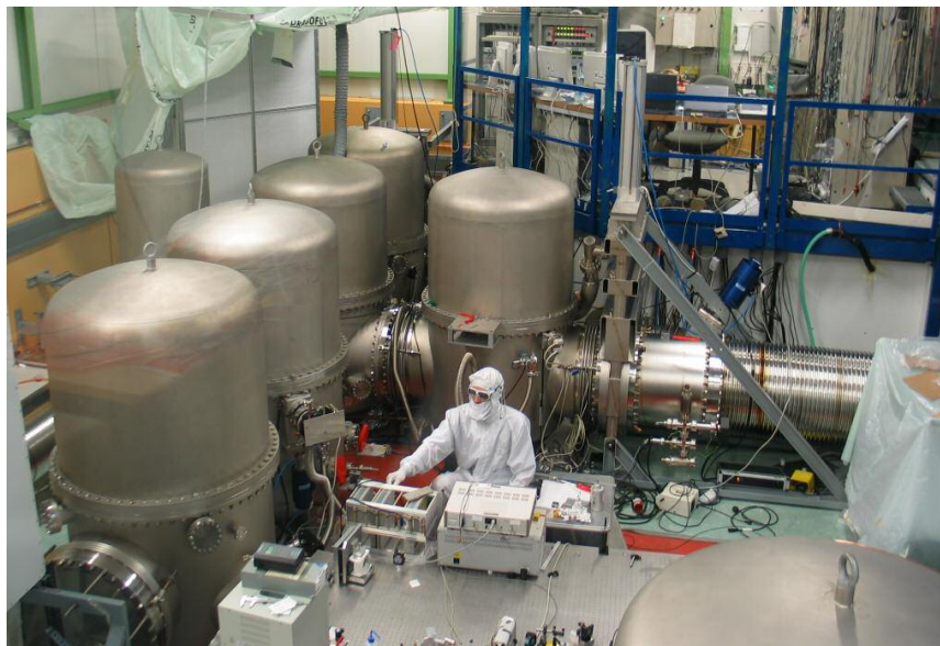
Fig. 3.10 – GEO600 vacuum system.
