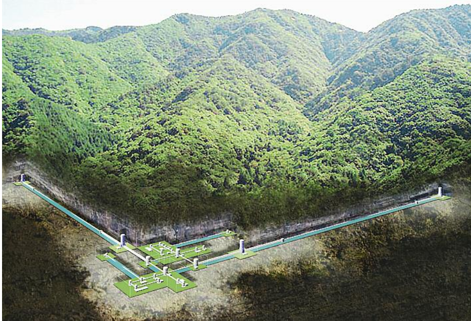
Fig. 5.4 – Artist’s impression of the LCGT detector, located underground at the Kamioka mine.
