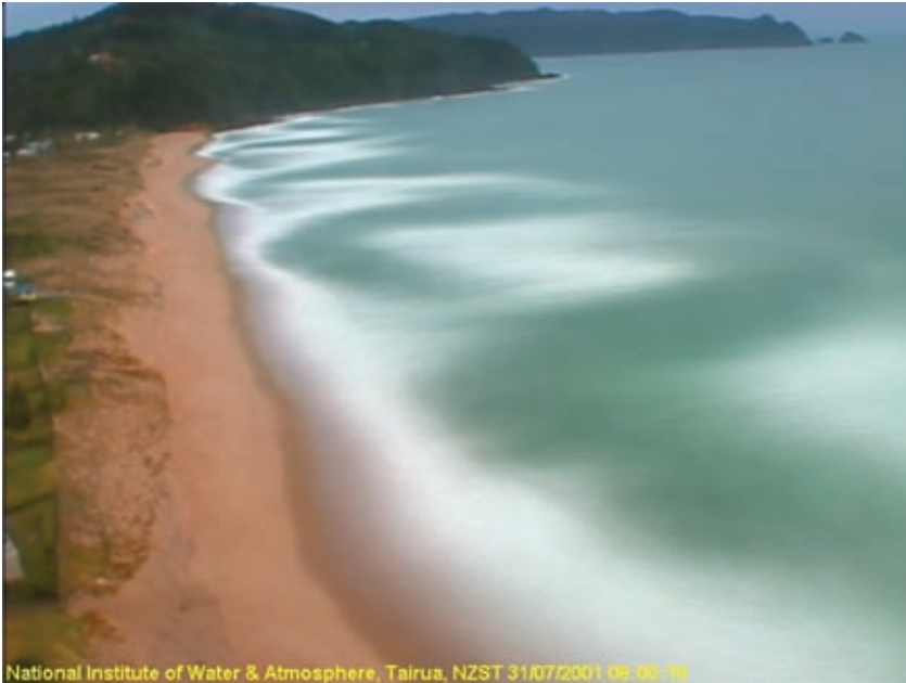
National Institute of Water & Atmosphere, Tairua, NZST 31/07/2001 08:00:10 An averaged video composite of numerous 1-second images of waves at Tairua Beach. The whitest areas indicate areas where wave breaking is dominant, and darker areas indicate surf rips, that channel water back out to sea.
