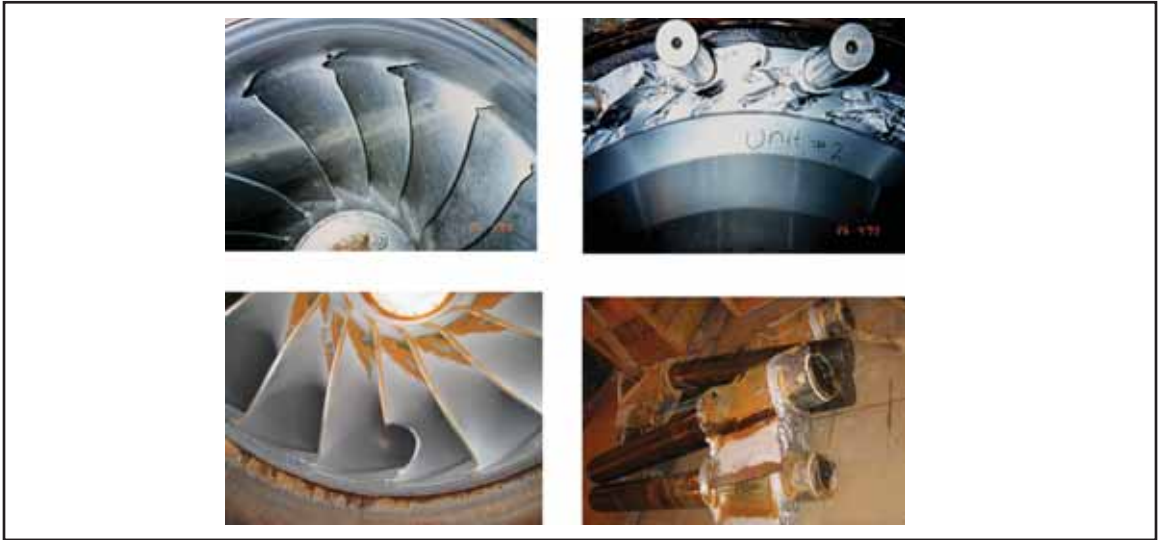
Figure 29: Sediment Induced wear of Hydro-turbine (Bishwakarma MB. 2008)
