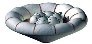
Soyuz Fregat upper stage entry configuration with IRDT flexible heatshield deployed (Image: ESA)
