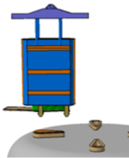
1. Move cask to the upper port
