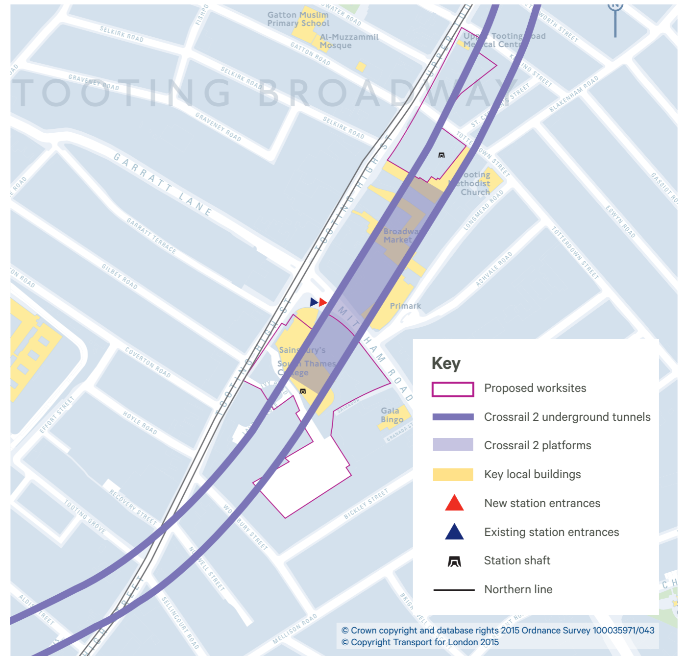
Worksites require to build Crossrail 2 at Tooting Broadway
