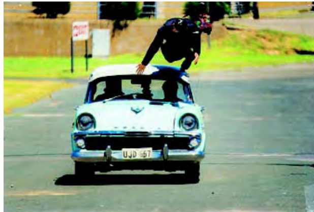
The dummy has just cleared the sun-visor and is being displaced to the left of the Holden.
