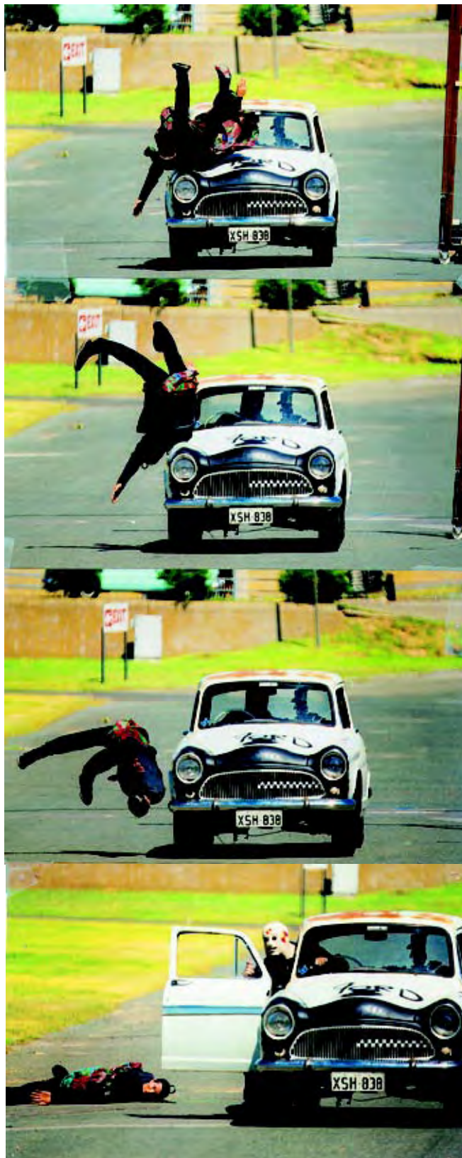
A sequence of four photos of a crash test with one of the Simcas. On this occasion the dummy was placed to be hit with the right side of the car to show that if it is hit right, it goes right, and if it is hit left, it goes left.
