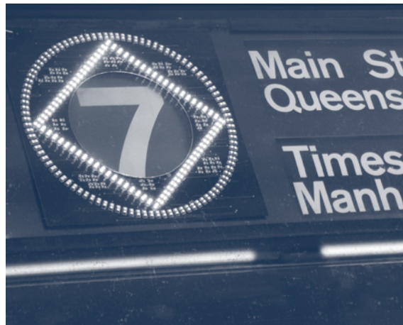
Electronic signage on the 7 line allows customers to distinguish local and express trains.
