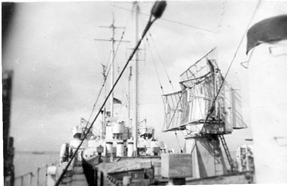
Antenna of AMES 11 back-up GCI radar on FDT 217
