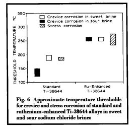
"cathode-modification". Of particular engineering value are the dramatic increases in the threshold temperatures for crevice corrosion and SCC offered by the ruthenium-enhanced Ti-38644 alloy in sweet and sour sodium chloride-rich brines (13), see Figure 6.
