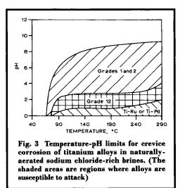
within acidic crevices. The enhanced crevice resistance of Ti-Ru alloys is essentially equivalent to that of Ti-Pd alloys, as indicated by the guidelines in Figure 3.
