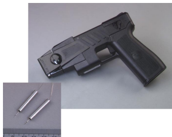
Taser showing barbed electrodes
