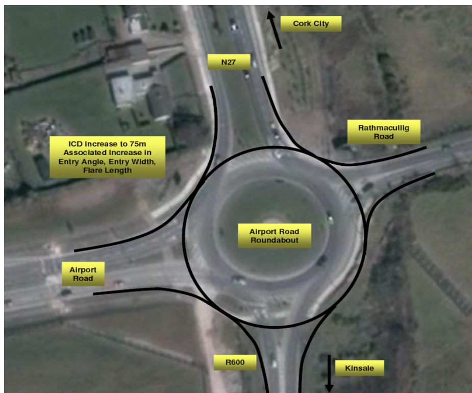
Figure 8-2: Geometric Junction Improvements – Airport Road Roundabout
