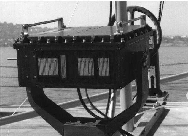
Figure 2. Photo of the transducer array face. The sparse array produces 28 spatial lags from 0 to 27 times the transducer spacing (roughly 0.98 cm each). (Photo by L. Green)
