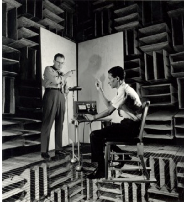
Fig. 2-6. Photograph of the anechoic chamber, or free-space room. A wire grid formed the floor. Manfred R. Schroeder is standing and James E. West is sitting as they perform acoustic measurements in this room without echoes and with perfect silence. [Photo courtesy of AT&T Archives and History Center.]
