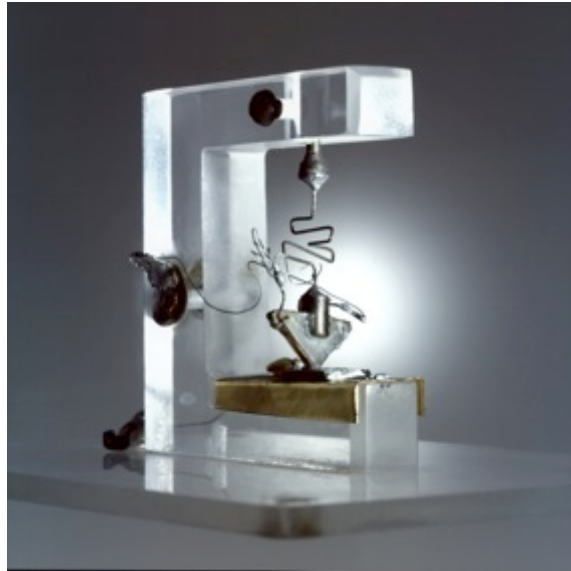
Fig. 5-1. The first transistor was a point-contact device (shown here), invented in 1947 at Bell Labs in Murray Hill by John Bardeen and Walter Brattain. The following year William Shockley conceived the bipolar junction transistor, and all three shared the Nobel Prize in Physics in 1956. [Photo of the original transistor courtesy of Alcatel-Lucent USA Inc. / Bell Labs.]
