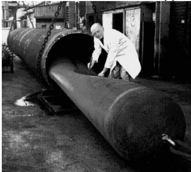
Figure 21: Photograph showing buckled linepipe section
